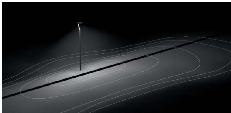
[A60] Asymmetric 'forward throw' distribution. Nominal angle of peak intensity through 60-65° from nadir (downward vertical). Rearward light spillage limited to an angle of 10°.
